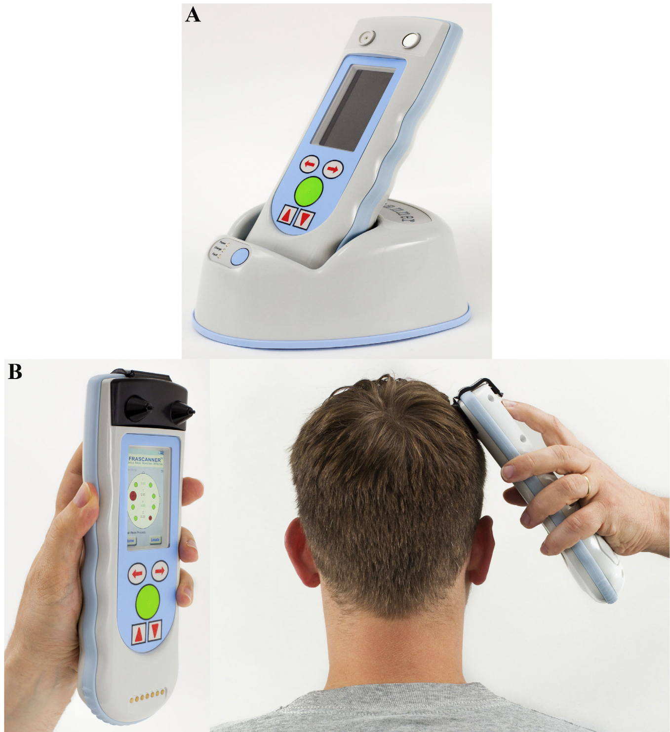
Fig. 2. Portable NIR detector of intracranial hemorrhage, the Infrascanner: (a) The scanner positioned inside the charging cradle, (b) The scanner with a disposable fiber optic shield in hand and placed on a head.
